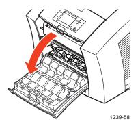
**2.** Remove the maintenance drawer from the printer. Once you've removed the maintenance drawer, keep it level.
